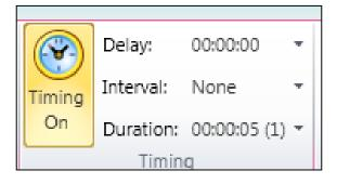
Users can then input the required kinetic parameters for a measurement cycle. The measurement cycle refers to the point of absorbance measurement including any timed delay and/or interval until the next reading.
