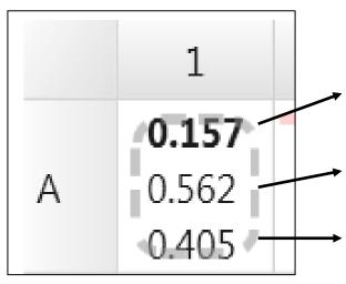
The bold value refers to the absorbance measurement after wavelength subtraction of the absorbance at the measurement wavelength from the absorbance at the reference wavelength.
