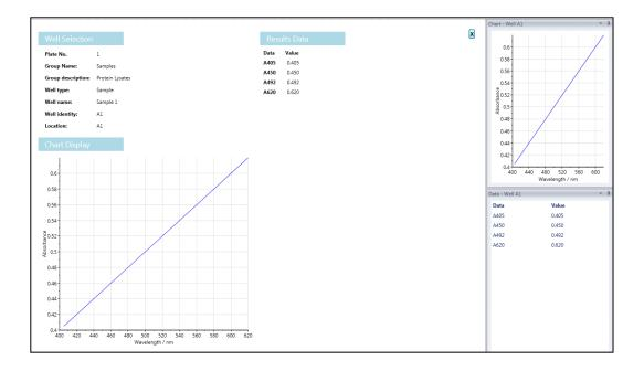
5. Results can be saved to 'Database'. A database is useful for saving, sharing and extracting data via communication with an external database system such as LIMS. Users can save files and templates onto the database, 'File' (save to own personal file), or 'Save Method Template' (saves the method protocol for future use).
